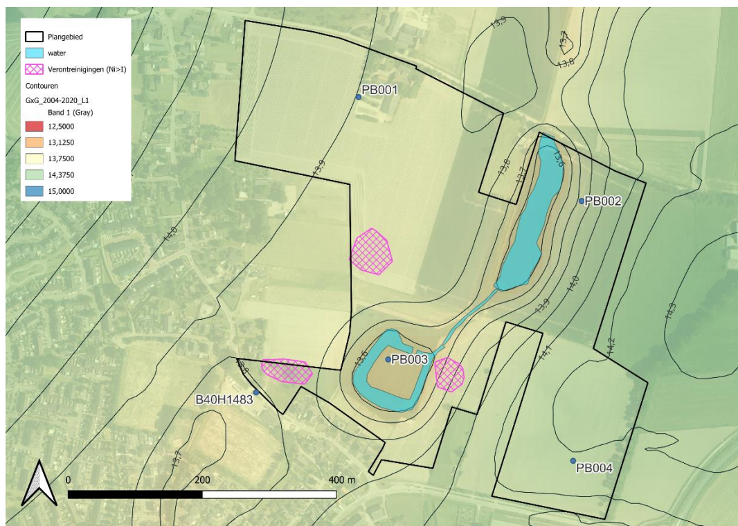
Figuur 4-4: Model GHG scenario 1 (modellaag 1).
